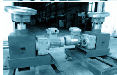
Example of combined application of screw jacks and reducer - Military equipment application
