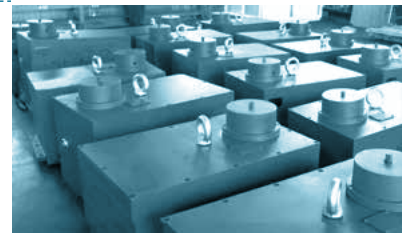
Vertical lifting box-Typical application of screw jacks on machine tools: Equipped with TR8010 screw, capable of lifting 250KN weight, used in pairs with strict synchronization requirements.
