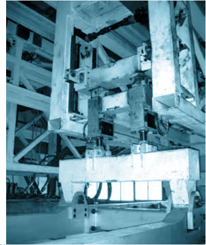
Screw Jacks application in large glass production line.
