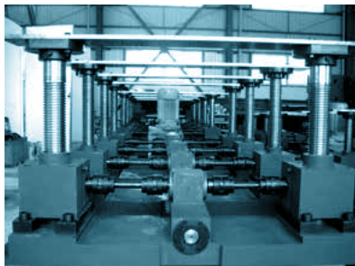
Application of screw jacks on large-scale water conservancy test benches: 50 meter long variable slope water tank, using screw jacks to achieve precise slope adjustment.
