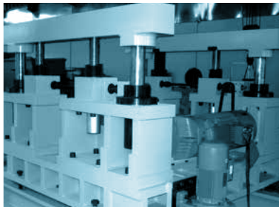
Screw jacks in large sheet metal production line applications: Lifting 54 tons Select 4 x CS250 Jacks + 2 x bevel gearboxes with Tr8010 screws
